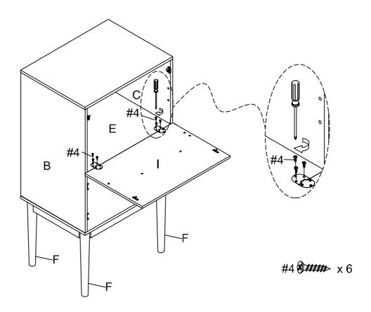
Step 12. Attach spring hinge (part #17) to left side panel (part B) and right side panel (part C) by using screws (part #4) and phillips head screwdriver.
